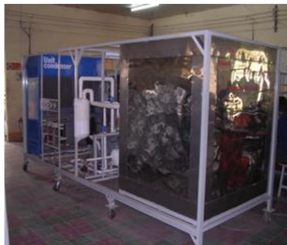
Figure 3b. The Refrigeration system DL-3 with the auto freezing (-45 ÷ -40) 0 C
