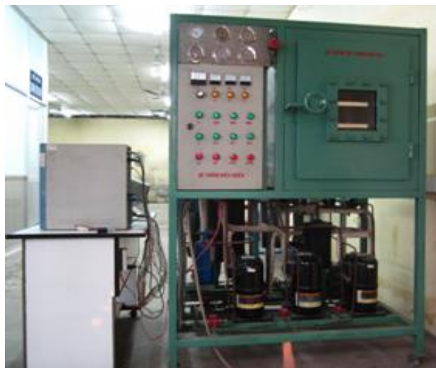
Figure 3a. The freeze drying system DS-3 with the auto-freezing (-50 ÷ -45) 0 C
