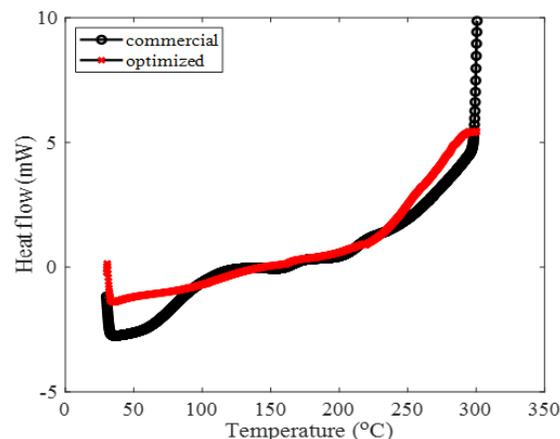
**Figure 9.** DSC Thermograms of commercial and optimized powder
