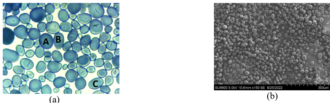
Figure 2. Arrowroot starch granule morphology under the (a) light microscope and (b) scanning electron microscope (A – Oval shape, B – Spherical shape, C – Irregular globular shape)
