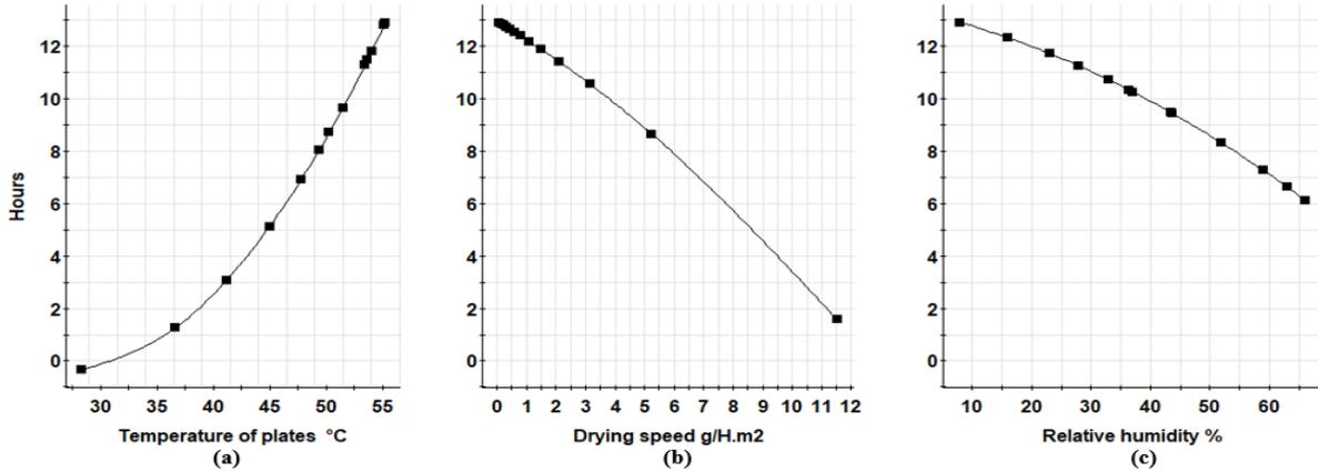
Figure 8. Drying time variation with experiment number 13
