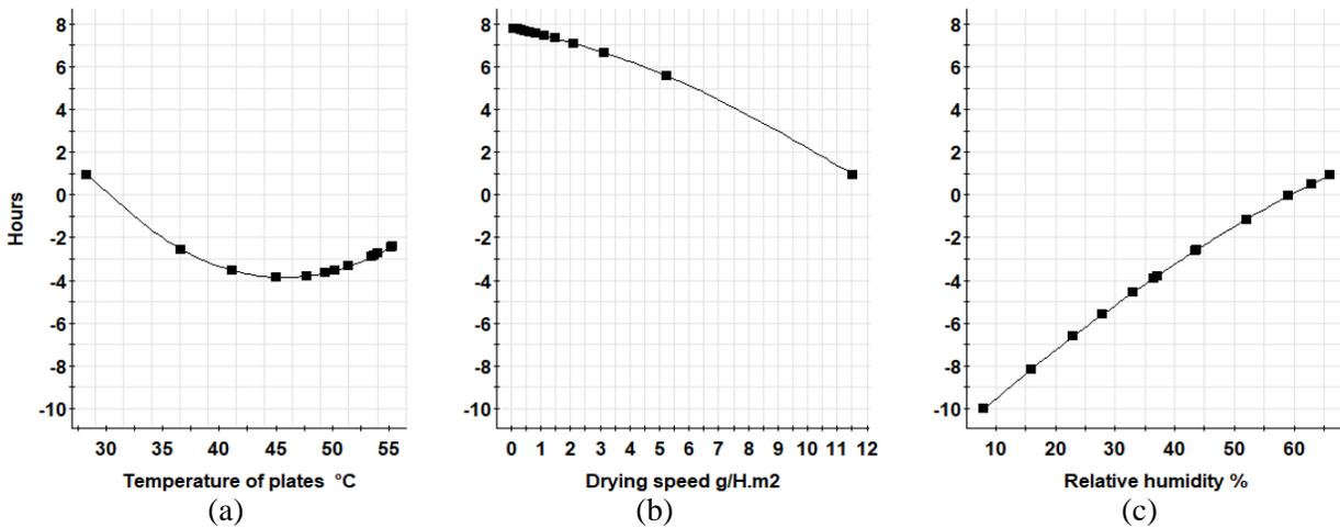
**Figure 6.** Drying time variation with experiment number 1
