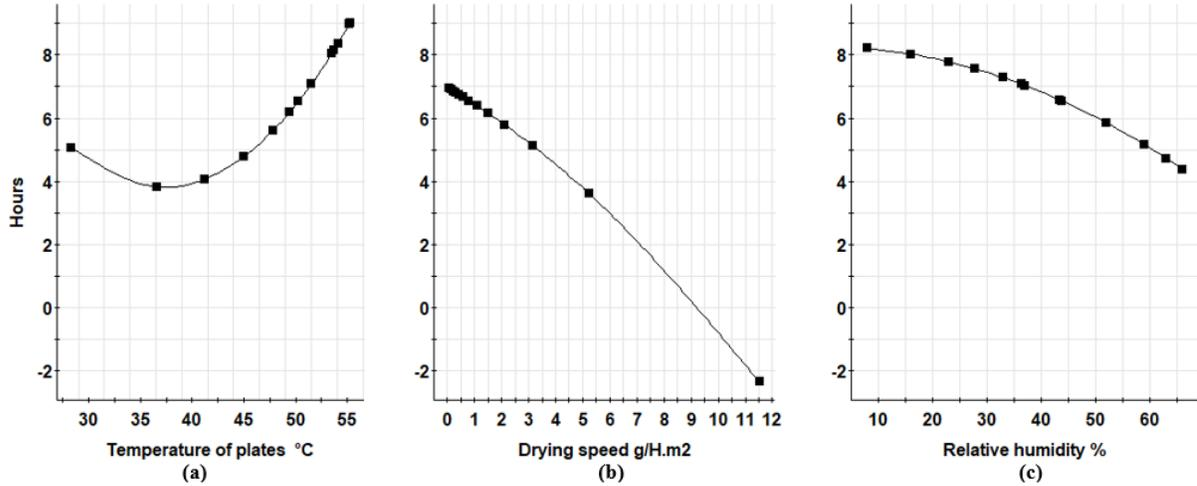
**Figure 7.** Drying time variation with experiment number 7
