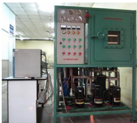
Figure 2. The freeze drying system DS-3 with the auto-freezing (-50 ÷ -45) 0 C
