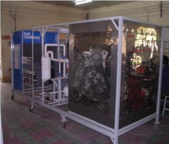
Fig 3. The Refrigeration system DL-3 with the auto freezing  $(-45 \div -40)^{\circ}\text{C}$
