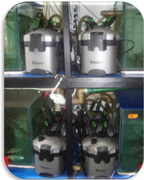
Figure 3. Water quality recirculation and conditioning equipment.
