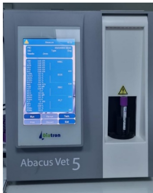
Figure 5. Hematology analyzer used to determine hematological parameters.
