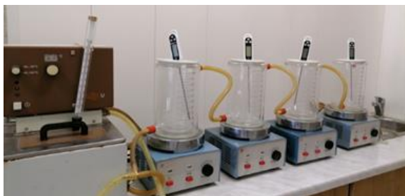
Figure 2. Bioreactor for thermally induced denaturation of whey protein
