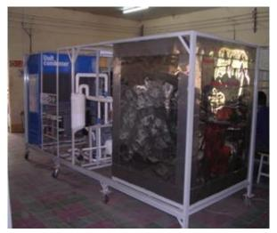
Fig 3. The Refrigeration system DL-3 with the auto freezing  $(-45 \div - 40)^{0}$ C
