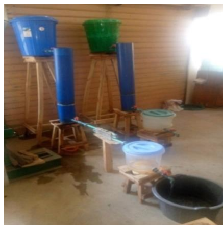
Figure 5. Pictorial view of the fabricated slow sand filters
