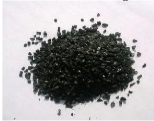
Figure 1. Granular activated carbon for the filter
