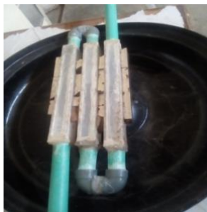
Figure 2. Pictorial view of neodymium magnet
