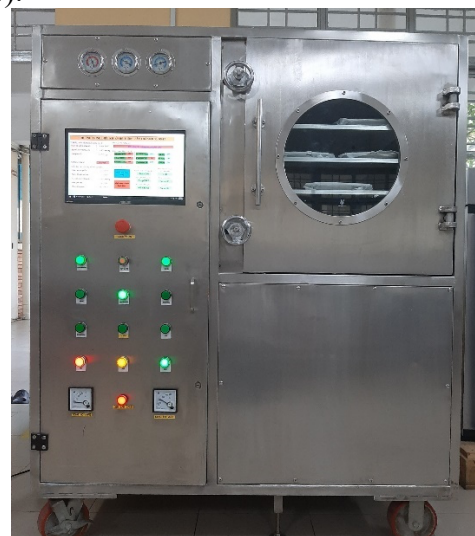
Figure 2. The DS-12 Freeze Drying System automatically measured and controlled by compute
